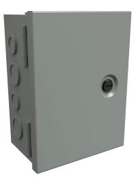
Hammond enclosure, NEMA 1, 30 x 24 x 6in (HxWxD), wall mount, with knockouts, carbon steel, ANSI 61 gray, powder coat finish, single-door, 1/4-turn flush-mounted latch.
