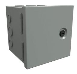
Hammond enclosure, NEMA 1, 24 x 24 x 6in (HxWxD), wall mount, with knockouts, carbon steel, ANSI 61 gray, powder coat finish, single-door, 1/4-turn flush-mounted latch.
