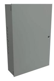
Hammond enclosure, NEMA 1, 18 x 12 x 4in (HxWxD), wall mount, with knockouts, carbon steel, ANSI 61 gray, powder coat finish, single-door, 1/4-turn flush-mounted latch.
