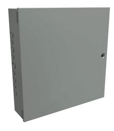
Hammond enclosure, NEMA 1, 16 x 12 x 4in (HxWxD), wall mount, with knockouts, carbon steel, ANSI 61 gray, powder coat finish, single-door, 1/4-turn flush-mounted latch.
