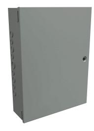
Hammond enclosure, NEMA 1, 12 x 12 x 6in (HxWxD), wall mount, with knockouts, carbon steel, ANSI 61 gray, powder coat finish, single-door, 1/4-turn flush-mounted latch.
