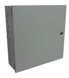
Hammond enclosure, NEMA 1, 12 x 12 x 4in (HxWxD), wall mount, with knockouts, carbon steel, ANSI 61 gray, powder coat finish, single-door, 1/4-turn flush-mounted latch.
