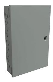
Hammond enclosure, NEMA 1, 12 x 10 x 4in (HxWxD), wall mount, with knockouts, carbon steel, ANSI 61 gray, powder coat finish, single-door, 1/4-turn flush-mounted latch.
