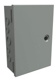
Hammond enclosure, NEMA 1, 10 x 8 x 6in (HxWxD), wall mount, with knockouts, carbon steel, ANSI 61 gray, powder coat finish, single-door, 1/4-turn flush-mounted latch.
