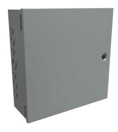
Hammond enclosure, NEMA 1,  $10 \times 10 \times 6$ in (HxWxD), wall mount, with knockouts, carbon steel, ANSI 61 gray, powder coat finish, single-door, 1/4-turn flush-mounted latch.
