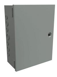
Hammond enclosure, NEMA 1, 10 x 10 x 4in (HxWxD), wall mount, with knockouts, carbon steel, ANSI 61 gray, powder coat finish, single-door, 1/4-turn flush-mounted latch.
