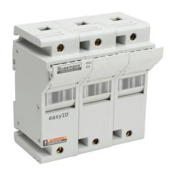
Bussmann modular fuse holder, accepts Class J fuses, 60A, 600 VAC/VDC or less, 3-pole, 18-1 AWG copper only, integral pressure plate with separate spade connection, 35mm DIN rail or panel mount. Package of 2.
