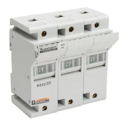
Bussmann modular fuse holder, with indicator, accepts Class J fuses, 60A, 600 VAC/VDC or less, 3-pole, 18-1 AWG copper only, integral pressure plate with separate spade connection, 35mm DIN rail or panel mount. Package of 2.
