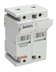
Bussmann modular fuse holder, accepts Class J fuses, 60A, 600 VAC/VDC or less, 2-pole, 18-1 AWG copper only, integral pressure plate with separate spade connection, 35mm DIN rail or panel mount. Package of 3.
