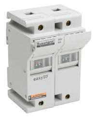
Bussmann modular fuse holder, with indicator, accepts Class J fuses, 60A, 600 VAC/VDC or less, 2-pole, 18-1 AWG copper only, integral pressure plate with separate spade connection, 35mm DIN rail or panel mount. Package of 3.
