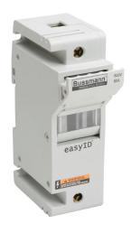
Bussmann modular fuse holder, accepts Class J fuses, 60A, 600 VAC/VDC or less, 1-pole, 18-1 AWG copper only, integral pressure plate with separate spade connection, 35mm DIN rail or panel mount. Package of 6.
