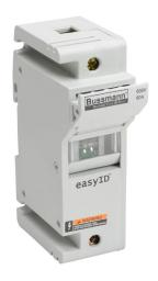
Bussmann modular fuse holder, with indicator, accepts Class J fuses, 60A, 600 VAC/VDC or less, 1-pole, 18-1 AWG copper only, integral pressure plate with separate spade connection, 35mm DIN rail or panel mount. Package of 6.
