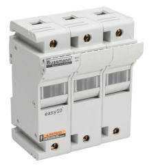
Bussmann modular fuse holder, accepts Class J fuses, 30A, 600 VAC/VDC or less, 3-pole, 18-1 AWG copper only, integral pressure plate with separate spade connection, 35mm DIN rail or panel mount. Package of 2.
