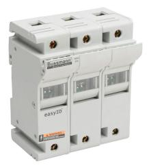
Bussmann modular fuse holder, with indicator, accepts Class J fuses, 30A, 600 VAC/VDC or less, 3-pole, 18-1 AWG copper only, integral pressure plate with separate spade connection, 35mm DIN rail or panel mount. Package of 2.
