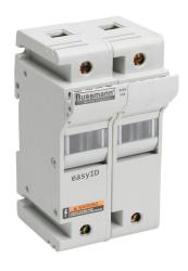
Bussmann modular fuse holder, accepts Class J fuses, 30A, 600 VAC/VDC or less, 2-pole, 18-1 AWG copper only, integral pressure plate with separate spade connection, 35mm DIN rail or panel mount. Package of 3.
