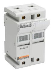
Bussmann modular fuse holder, with indicator, accepts Class J fuses, 30A, 600 VAC/VDC or less, 2-pole, 18-1 AWG copper only, integral pressure plate with separate spade connection, 35mm DIN rail or panel mount. Package of 3.
