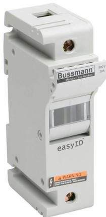
Bussmann modular fuse holder, accepts Class J fuses, 30A, 600 VAC/VDC or less, 1-pole, 18-1 AWG copper only, integral pressure plate with separate spade connection, 35mm DIN rail or panel mount. Package of 6.
