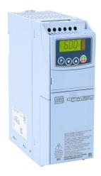
WEG Electric CFW320 series AC general purpose drive, enclosed, 230 VAC, 3hp with 3-phase and 1-phase input, SVC, V/Hz or VVW mode, B frame, integrated dynamic braking. Optional communication and I/O modules available.
