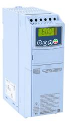
WEG Electric CFW320 series AC general purpose drive, enclosed, 460 VAC, 5hp with 3-phase input, SVC, V/Hz or VVW mode, B frame, integrated dynamic braking. Optional communication and I/O modules available.
