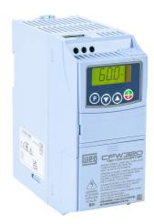
WEG Electric CFW320 series AC general purpose drive, enclosed, 230 VAC, 1-1/2hp with 1-phase input, SVC, V/Hz or VVW mode, A frame. Optional communication and I/O modules available.
