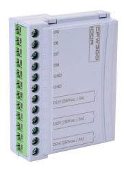
WEG Electric CFW300 series discrete combo module, Input: 4-point, 24 VDC, sinking/sourcing, Output: 3-point, 250 VAC, relay, (3) Form A (SPST) relays, 5A/point. For use with WEG CFW300 series AC drives.
