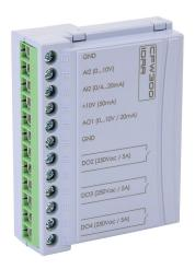
WEG Electric CFW300 series relay/analog combo module, Analog Input: 1-channel, current/voltage, Analog Output: 1-channel, current/voltage, Discrete Output: 3-point, relay, (3) Form A (SPST) relays. For use with WEG CFW300 series AC drives.
