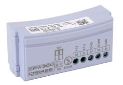
WEG Electric CFW300 series communication module, Modbus RTU, 2 ports, (1) RS-485 (5-pin terminal) and (1) miniB-USB port(s). For use with WEG CFW300 series AC drives.
