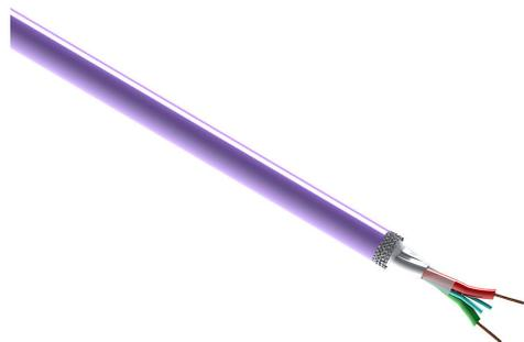
igus continuous flexing Profibus cable, shielded, AWM, 1 twisted pair, 24 AWG (0.25mm<sup>2</sup>), bare copper, TPE conductor insulation material, red and green, PVC jacket, purple, cut to length.
