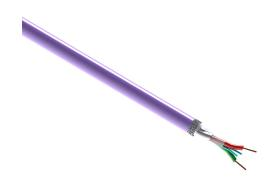
igus continuous flexing Profibus cable, shielded, AWM, 1 twisted pair, 24 AWG (0.25mm2), bare copper, TPE conductor insulation material, red and green, PVC jacket, purple, cut to length.
