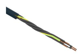
igus continuous flexing control cable, unshielded, 5 conductors (includes ground), 14 AWG (2.50mm2), bare copper, TPE conductor insulation material, black with white numbers and green/yellow ground, TPE jacket, gray, cut to length.
