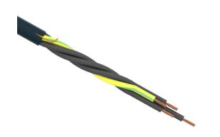
igus continuous flexing control cable, unshielded, 4 conductors (includes ground), 14 AWG (2.50mm2), bare copper, TPE conductor insulation material, black with white numbers and green/yellow ground, TPE jacket, gray, cut to length.
