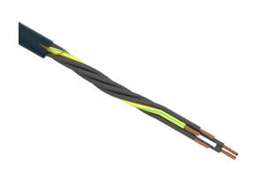
igus continuous flexing control cable, unshielded, 5 conductors (includes ground), 16 AWG (1.50mm2), bare copper, TPE conductor insulation material, black with white numbers and green/yellow ground, TPE jacket, gray, cut to length.
