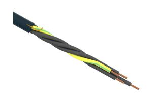
igus continuous flexing control cable, unshielded, 4 conductors (includes ground), 16 AWG (1.50mm2), bare copper, TPE conductor insulation material, black with white numbers and green/yellow ground, TPE jacket, gray, cut to length.
