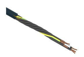
igus continuous flexing control cable, unshielded, 7 conductors (includes ground), 18 AWG (0.75mm2), bare copper, TPE conductor insulation material, black with white numbers and green/yellow ground, TPE jacket, gray, cut to length.
