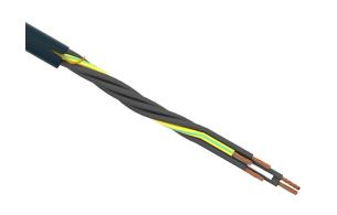
igus continuous flexing control cable, unshielded, 5 conductors (includes ground), 18 AWG (0.75mm2), bare copper, TPE conductor insulation material, black with white numbers and green/yellow ground, TPE jacket, gray, cut to length.
