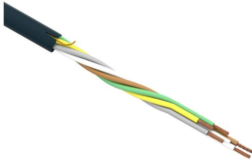
igus continuous flexing control cable, unshielded, 5 conductors (includes ground), 20 AWG (0.50mm<sup>2</sup>), bare copper, TPE conductor insulation material, black with white numbers and green/yellow ground, TPE jacket, gray, cut to length.
