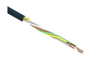
igus continuous flexing control cable, unshielded, 5 conductors (includes ground), 20 AWG (0.50mm2), bare copper, TPE conductor insulation material, black with white numbers and green/yellow ground, TPE jacket, gray, cut to length.
