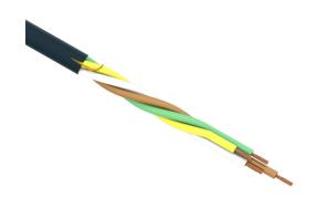
igus continuous flexing control cable, unshielded, 4 conductors (includes ground), 20 AWG (0.50mm2), bare copper, TPE conductor insulation material, black with white numbers and green/yellow ground, TPE jacket, gray, cut to length.
