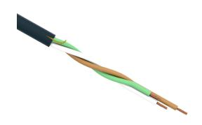
igus continuous flexing control cable, unshielded, 3 conductors (includes ground), 20 AWG (0.50mm2), bare copper, TPE conductor insulation material, black with white numbers and green/yellow ground, TPE jacket, gray, cut to length.
