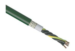
igus continuous flexing control cable, shielded, 4 conductors (includes ground), 14 AWG (2.50mm2), bare copper, PVC conductor insulation material, black with white numbers and green/yellow ground, PVC jacket, green, cut to length.
