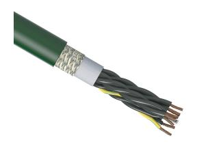
igus continuous flexing control cable, shielded, 12 conductors (includes ground), 16 AWG (1.50mm2), bare copper, PVC conductor insulation material, black with white numbers and green/yellow ground, PVC jacket, green, cut to length.
