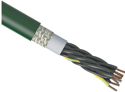
igus continuous flexing control cable, shielded, 12 conductors (includes ground), 16 AWG (1.50mm<sup>2</sup>), bare copper, PVC conductor insulation material, black with white numbers and green/yellow ground, PVC jacket, green, cut to length.
