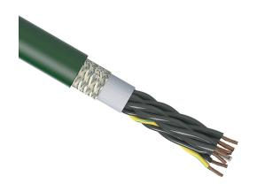
igus continuous flexing control cable, shielded, 12 conductors (includes ground), 16 AWG (1.50mm2), bare copper, PVC conductor insulation material, black with white numbers and green/yellow ground, PVC jacket, green, cut to length.
