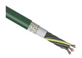
igus continuous flexing control cable, shielded, 7 conductors (includes ground), 16 AWG (1.50mm2), bare copper, PVC conductor insulation material, black with white numbers and green/yellow ground, PVC jacket, green, cut to length.
