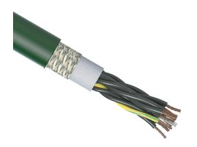
igus continuous flexing control cable, shielded, 12 conductors (includes ground), 18 AWG (0.75mm2), bare copper, PVC conductor insulation material, black with white numbers and green/yellow ground, PVC jacket, green, cut to length.
