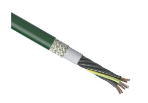
igus continuous flexing control cable, shielded, 7 conductors (includes ground), 18 AWG (0.75mm2), bare copper, PVC conductor insulation material, black with white numbers and green/yellow ground, PVC jacket, green, cut to length.
