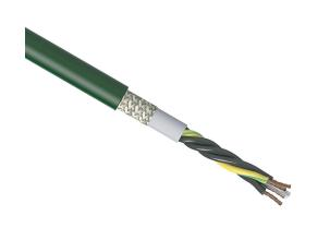
igus continuous flexing control cable, shielded, 4 conductors (includes ground), 18 AWG (0.75mm2), bare copper, PVC conductor insulation material, black with white numbers and green/yellow ground, PVC jacket, green, cut to length.
