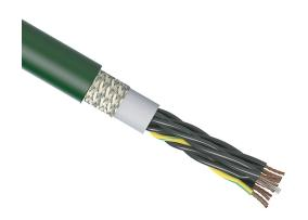
igus continuous flexing control cable, shielded, 12 conductors (includes ground), 20 AWG (0.50mm2), bare copper, TPE conductor insulation material, black with white numbers and green/yellow ground, PVC jacket, green, cut to length.
