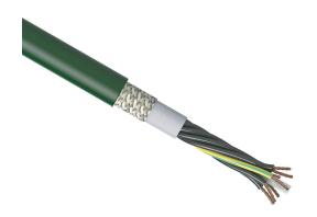
igus continuous flexing control cable, shielded, 7 conductors (includes ground), 20 AWG (0.50mm2), bare copper, TPE conductor insulation material, black with white numbers and green/yellow ground, PVC jacket, green, cut to length.
