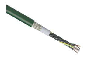
igus continuous flexing control cable, shielded, 5 conductors (includes ground), 20 AWG (0.50mm2), bare copper, TPE conductor insulation material, black with white numbers and green/yellow ground, PVC jacket, green, cut to length.
