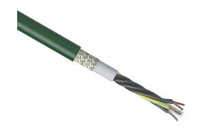
igus continuous flexing control cable, shielded, 5 conductors (includes ground), 20 AWG (0.50mm2), bare copper, TPE conductor insulation material, black with white numbers and green/yellow ground, PVC jacket, green, cut to length.
