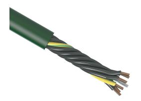
igus continuous flexing control cable, unshielded, 7 conductors (includes ground), 14 AWG (2.50mm2), bare copper, PVC conductor insulation material, black with white numbers and green/yellow ground, PVC jacket, green, cut to length.
