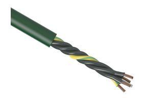
igus continuous flexing control cable, unshielded, 4 conductors (includes ground), 14 AWG (2.50mm2), bare copper, PVC conductor insulation material, black with white numbers and green/yellow ground, PVC jacket, green, cut to length.
