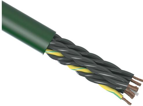
igus continuous flexing control cable, unshielded, 12 conductors (includes ground), 16 AWG (1.50mm<sup>2</sup>), bare copper, PVC conductor insulation material, black with white numbers and green/yellow ground, PVC jacket, green, cut to length.
