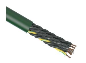
igus continuous flexing control cable, unshielded, 12 conductors (includes ground), 16 AWG (1.50mm2), bare copper, PVC conductor insulation material, black with white numbers and green/yellow ground, PVC jacket, green, cut to length.
