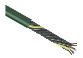
igus continuous flexing control cable, unshielded, 7 conductors (includes ground), 16 AWG (1.50mm2), bare copper, PVC conductor insulation material, black with white numbers and green/yellow ground, PVC jacket, green, cut to length.
